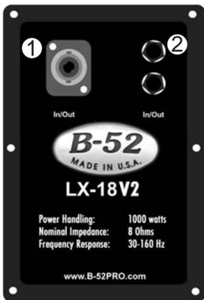
The LX-18V2 includes (2) 1/4" phone jacks and one Neutrik NL4 Speakon input terminals. All three terminals are internally connected in parallel. Each of the three connections can be used as an input or as an output.
