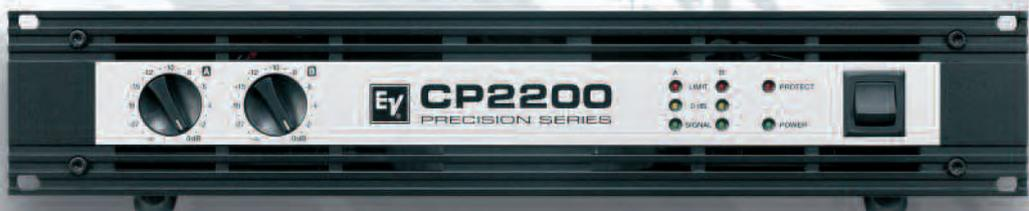
With up to 2 x 1100 watts into 2 Ohms and 2 x 800 watts into 4 Ohms, the CP 2200 is not only a perfect complement to many full-range speaker cabinets, but also mid- and hi-frequency components in larger concert-sound systems. The CP 2200 utilizes a conventional transformer power supply, but still weighs only 16 kilograms.
