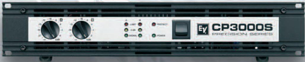
The lightweight workhorse of CP Series performs with 2 x 1600 watts into 2 Ohms and 2 x 1100 watts into 4 Ohms load — at only 8.15 kg in weight due to its switch mode power supply. Its reliability, coupled with its pleasing, rich sound makes it the first choice for high power full-range and mid/hi-cabinets.
