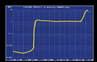
The THD of the amplifier is limited to a maximum of 1% for signals up to +21dBu. Even if overdriven, the amplifier will not create any objectionable "clipping signal effects" that are so fatal to speaker components.
