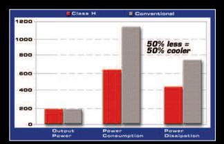
A conventional amplifier design has nearly double the power consumption and requires double the power dissipation of EV's Class-H design for equivalent output power. The Precision Series™ Compact Amplifier runs much cooler even under adverse conditions.
