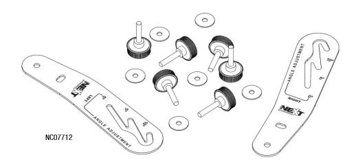
This kit can be applied connecting the PXH64/PXH95 to the PXA8001 power-rack, or connecting the PXH64/PXH95 to PXL118 SUB2. The assembly method is exactly the same, so we'll review only the assembly for a frontward tilt between the PXH64/PXH95 and the PXA8001.
