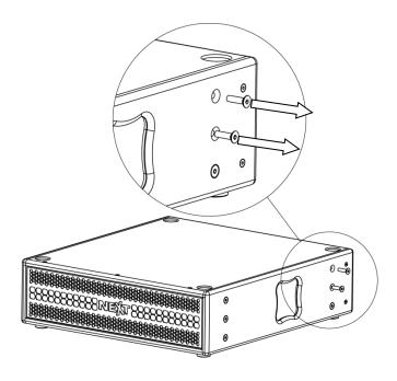
**Step 2.** – Remove the screw on the PXH64/PXH95 rear group as shown in the image.
