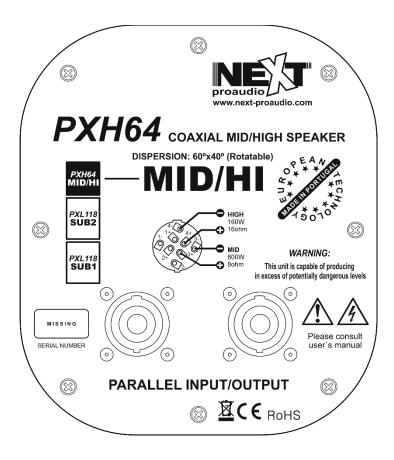
The 8 pins of the 2xNL8 SpeakON sockets are parallel wired within the enclosure. Either connector can be used to connect to the PXA8001 or another Subwoofer (PXL118 SUB1 or PXL118 SUB2).
