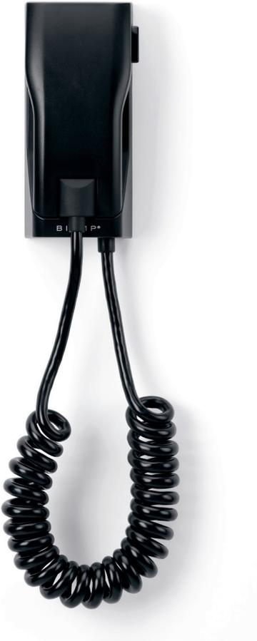
The Vocia Auxiliary Microphone 1 (VAM-1) device is an independent microphone assembly that functions as a slave device to the Vocia Wall and Desk Station (WS-4/10 and DS-4/10) series microphones and to the Vocia Input 6 (VI-6) for paging via the Paging Ports. Up to four VAM-1 slave microphones can be connected per VI-6.
