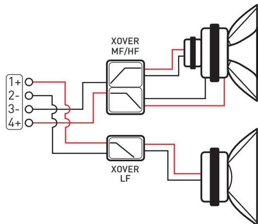
For single-channel amplification (mono-amp) it's necessary to make a cable bridge between the two poles (1+ to 4+ and 2- to 3-).
