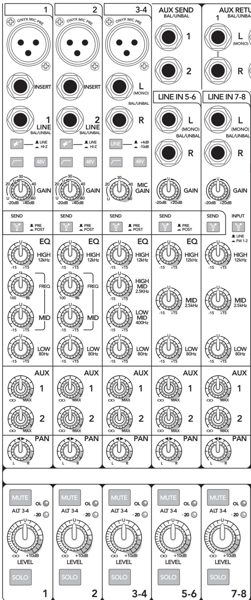
The vertical channel strips look very similar, and have only a few differences between them. Each channel works independently, and just controls the signals plugged into the inputs directly above it.
