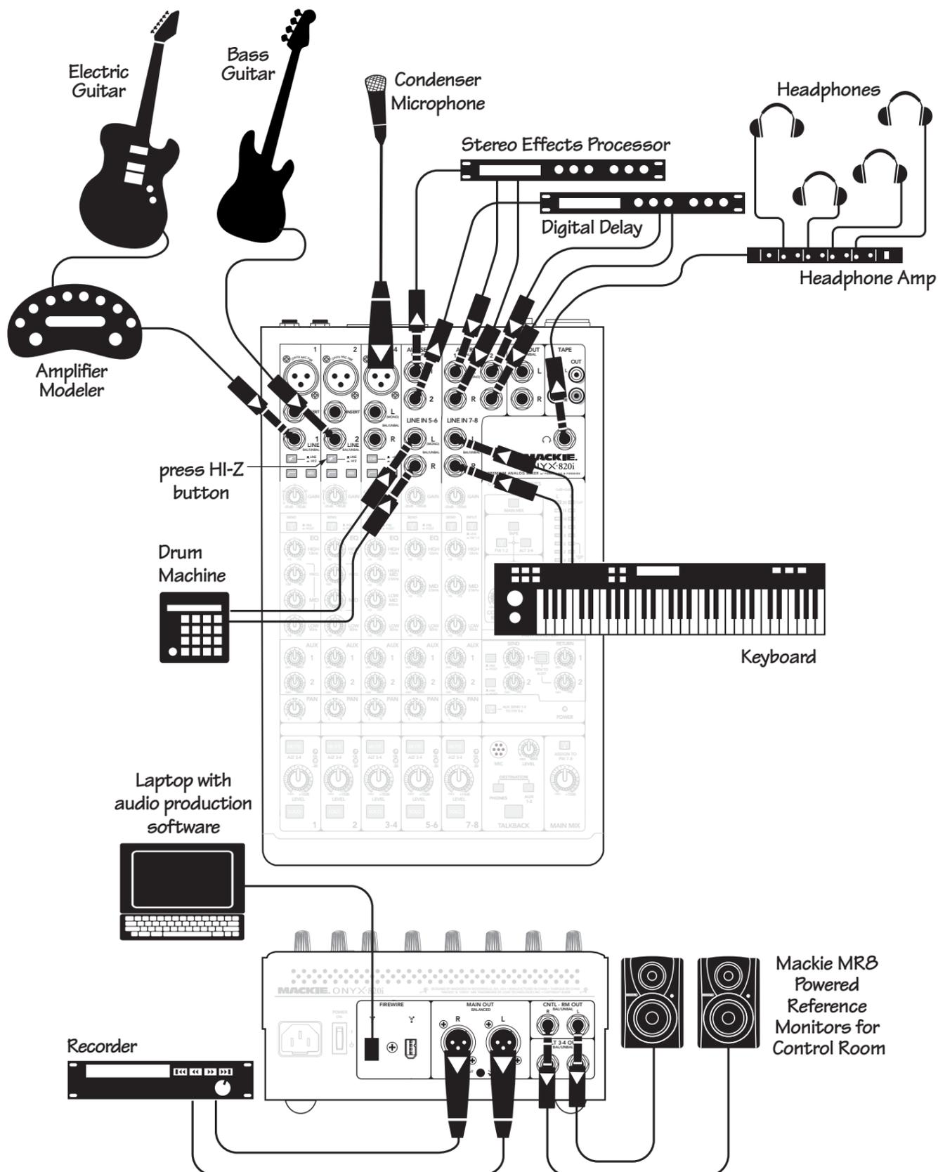
This diagram shows an electric guitar connected to an amplifier modeler, whose balanced line-level output is connected to the channel 1 line input, a bass guitar connected directly to the channel 2 input (with the hi-z switch engaged), a condenser microphone on channel 3/4 with phantom power engaged, a drum machine connected to channel 5/6, and a keyboard connected to channel 7/8. A headphone amplifier allows for multiple headphone use.
