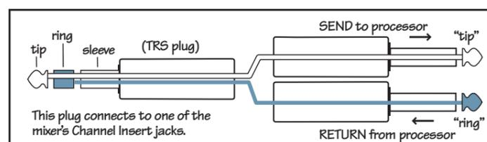
Insert jacks can be used as channel direct outputs; post-gain, and pre-EQ. See the connector section on page 30 (figure G) showing three ways to use insert cables.
