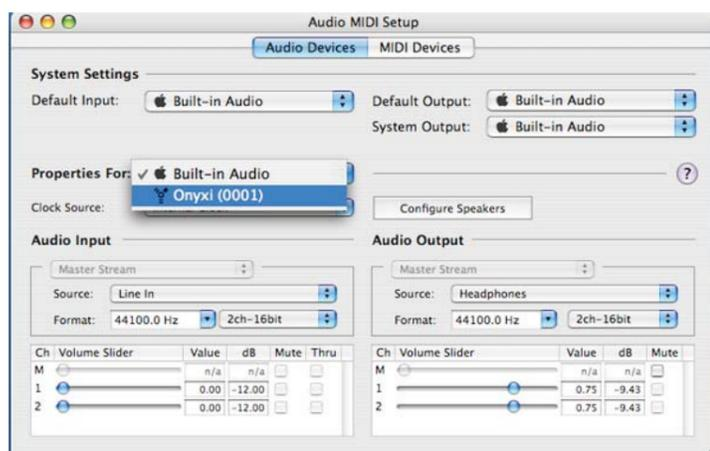
5. Here you can see the settings for the mixer. You can also choose it as your default input or output, as well as designate it to be used for system sound output. There are 8 channels of audio input from the Onyx 820i, and 2 channels of audio output to the Onyx 820i.
