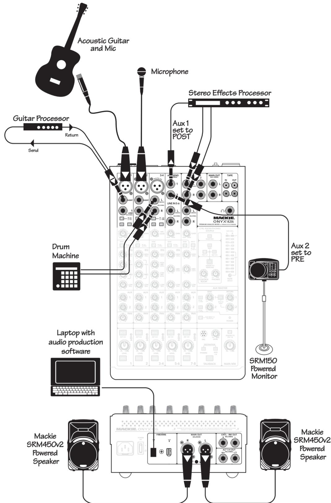
This diagram shows an acoustic guitar mic'd up directly to channel 1 and a microphone connected to channel 2 for vocals. A guitar processor is connected to the insert jack of channel 1.
