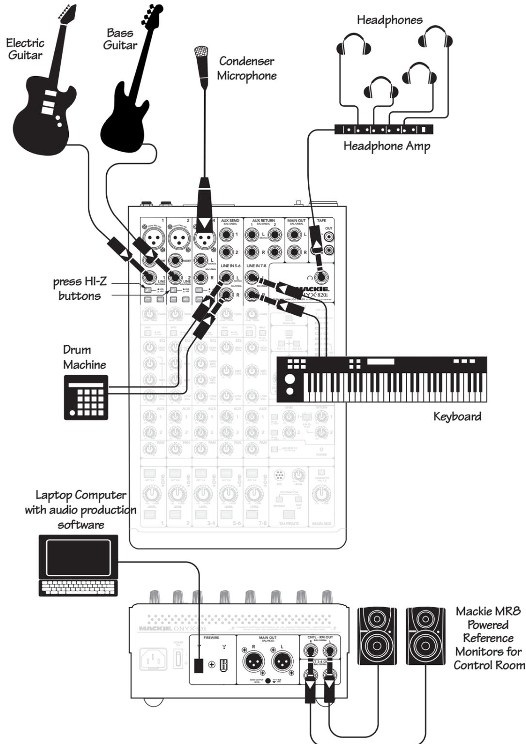
This diagram shows an electric guitar connected directly to channel 1 (with the hi-z switch engaged), a bass guitar connected directly to channel 2 (also with the hi-z engaged), a condenser microphone on channel 3/4 with the phantom power engaged, a drum machine connected to channel 5/6, and a keyboard connected to channel 7/8. A headphone amplifier allows for multiple headphone use during the recording process.
