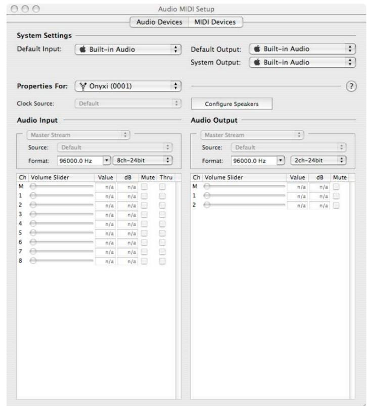
6. The Sample Rate is also shown from 44.1 kHz, 48 kHz, 88.2 kHz and 96 kHz.
