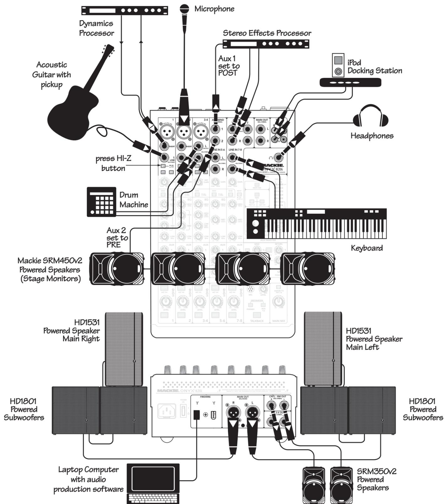
This diagram shows an acoustic-electric guitar connected to the channel 1 input (with the hi-z switch pressed down), a microphone connected to the channel 2 mic input, a drum machine connected to channel 3-4, and a keyboard connected to channel 7-8. Engage the +4dBu/-10dBV switch on channels 3-4 if your drum machine runs at -10 dBV. An iPod® can be used for intermission music.
