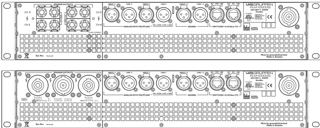
The PLM 10000Q is available with either binding posts or an “embedded patch panel” with Neutrik speakON connectors (2 x NLT4 and 1 x NLT8). Common connectors include; 2 x analog input XLR with switchable Iso-Float, 2 channels of AES/EBU with link-through capability for daisy chaining, 2 x EtherCON® for linking or redundancy. A 32 amp PowerCON® connector is used for mains supply.
