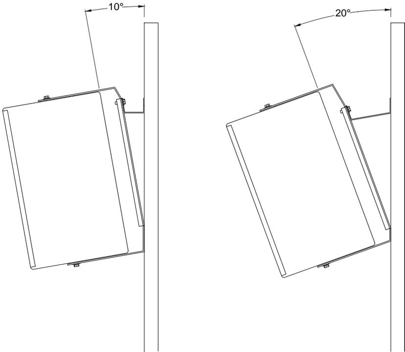
Optional standoffs are included with V SERIES Yoke Mounting Brackets to achieve a 10° or 20° downward or upward vertical tilt if desired.
