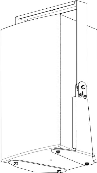
*Vertical Yoke kits for large V SERIES loudspeaker models V2-12, V2-15, V2-32 and V2-35 include left and right bottom yoke brackets.*
