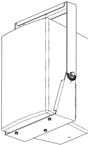
*Vertical Yoke kits for compact V SERIES loudspeaker models V2-6, V2-8, V2-26 and V2-28 include a single bottom U-bracket.*
