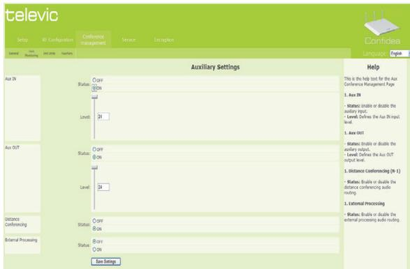
Activating the external processing allows to add external signal processing equipment or a mixing board.
