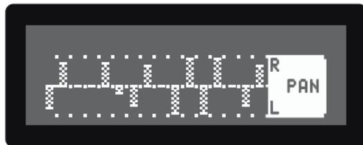
The Pan page allows you to adjust each channel's pan setting. The Pan page can be accessed by pressing the **<PAN>** button.
