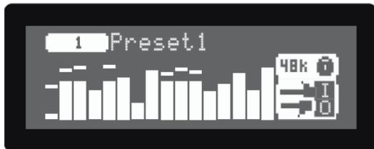
This is the first page visible on the PMC16's LCD display after boot up. The Meters page allows you to see the input level meters for all 16 input channels. The Meters page can be accessed by pressing the **<BACK>** button until the Meters page is displayed.
