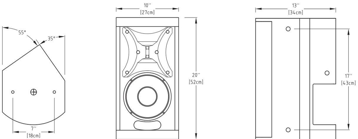
⊕ = Center of Gravity   ○ = M10 Threaded Rigging Point
