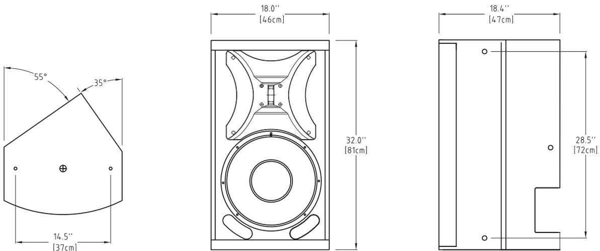
⊕ = Center of Gravity   ○ = M10 Threaded Rigging Point
