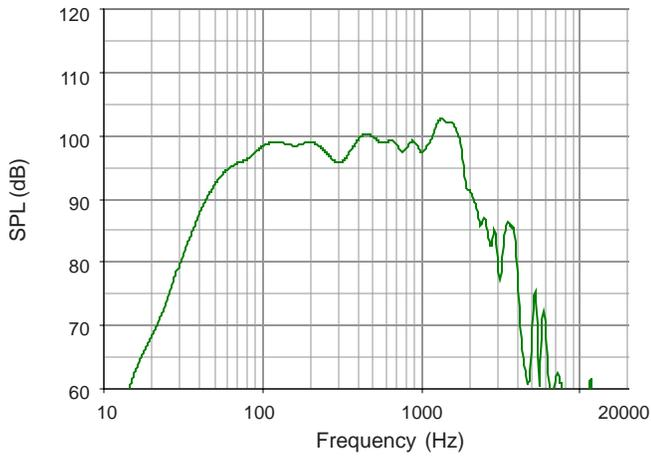
**Frequency Response: Digital Signal Processor**
