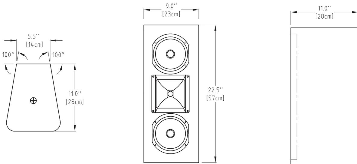
⊕ = Center of Gravity    ⊙ = 5/16" -18 Threaded Rigging Point
