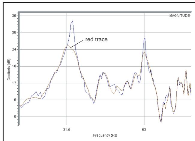
Figure 1: The magnitude vs frequency in the boathouse shows very strong resonant peaks. The red trace is with a single E-Trap™ tuned to two frequencies and turned on.
